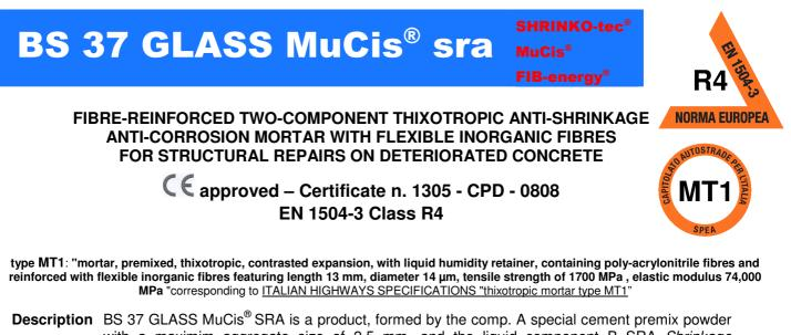
with a maximim aggregate size of 2.5 mm, and the liquid component B SRA Shrinkage Reducing Agent.
